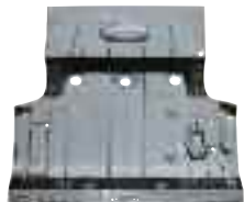
One Piece Trunk Floor Assembly
