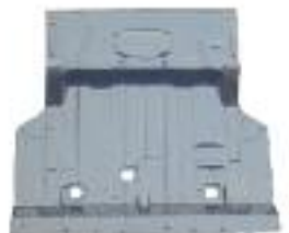
Trunk Floor Complete Assembly
